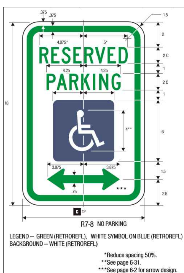
9 HANDICAP PARKING SIGN C16 NOT TO SCALE
